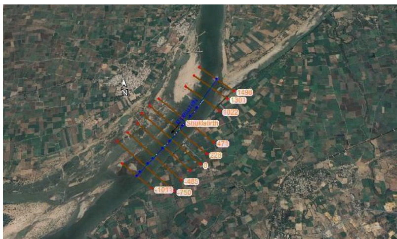
Fig-52: HEC-RAS model setup for Shuklatirth Site
